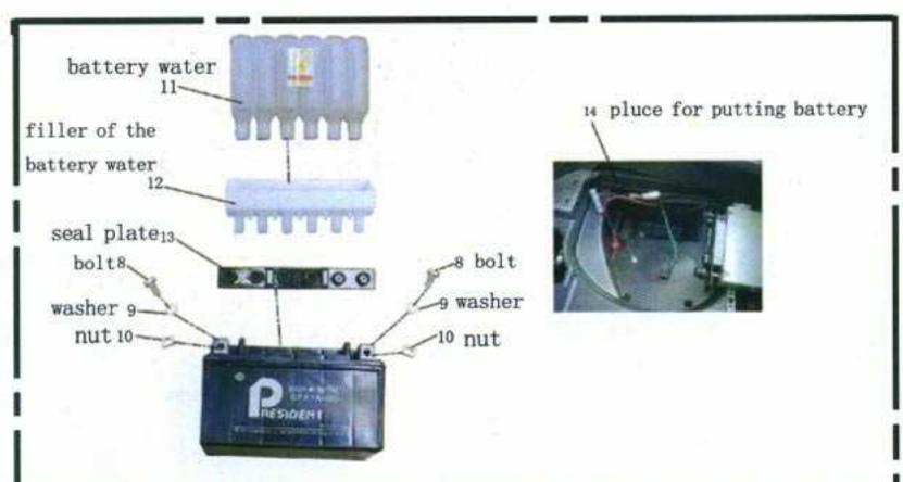
1. put filler (12) on the battery. 2. put the battery water (11) on the filler, press hard. 3. after put all the watter into the battery, put the seal plate(13) on the battery. 4. connect the positive pole of scooter and battery, connect the cathode of scooter and battery, use bolt(8) washer(9) and nut(10) to fix well.
